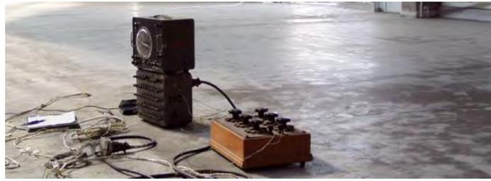
**Fig. 4. – Determination of forced displacements in slabs on ground**
