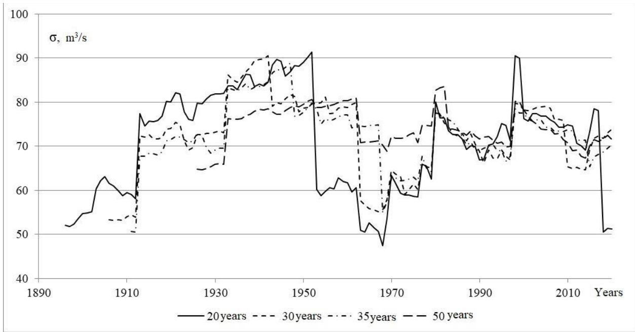
Figure 6 – Dynamics of moving dispersions for different periods of averaging the open channel minimum runoff of the Pripjat River at the Mozyr gauging station
