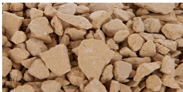
Figure 1 – Pink limestone natural coarse aggregate
