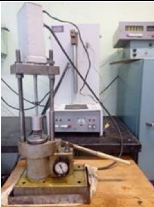
Figure 5 – Experimental setup for ultrasonic powder pressing
