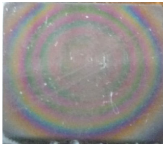
Figure 1 – The Sample with plotted thin-film silicium of containing coverages. Material of substructure WC-Co, the polished surface
