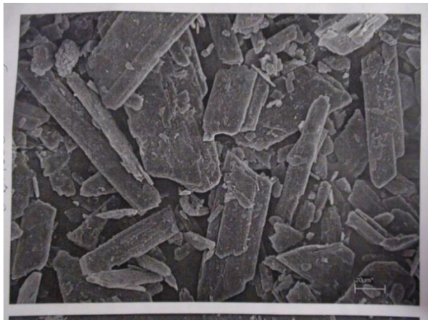
Figure 4 – Micrograph of the coarse fraction (from the cyclone) of dried PhG. Magnification 1000x
