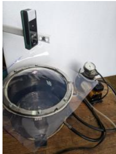
Figure 8 – Test bench for the bubble inflation test of the film sample
