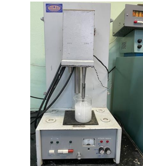
Figure 3 – Laboratory setup for ultrasonic mechanoactivation
