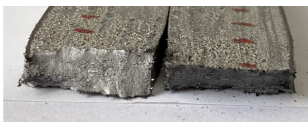
f – destruction cross-section (sample 6a)
