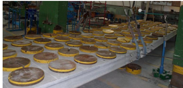
Figure 5 – Experimental investigation of the fragment of the hollow-core slabs [25]
