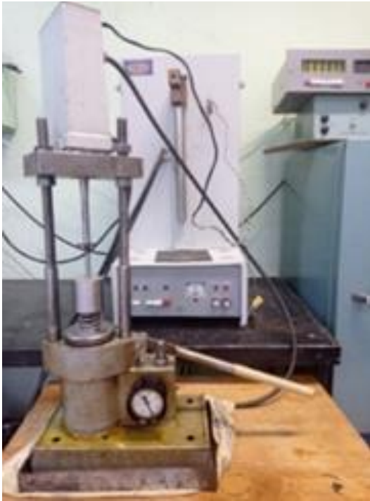
Figure 5 – Experimental setup for ultrasonic powder pressing
