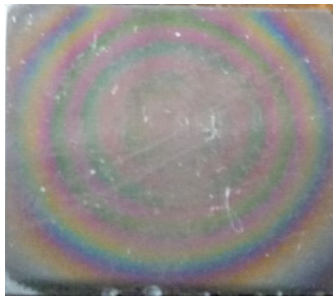
Figure 1 – The Sample with plotted thin-film silicon of containing coverages. Material of substructure WC-Co, the polished surface
